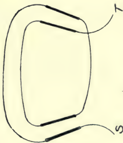
FIG. 207.—Typical Two-turn Coil.
